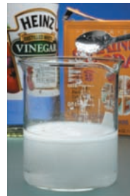
Baking soda Reacts with vinegar to form carbon dioxide and water, absorbing heat during the reaction.
